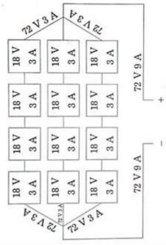
Given Potential difference is 18 V and current is 3A. The requirement is potential difference of 72 V and current is 9A Voltage remains the same if connected in parallel and gets added it they are connected in series. Current remains the same if connected in series but adds if connected in parallel
